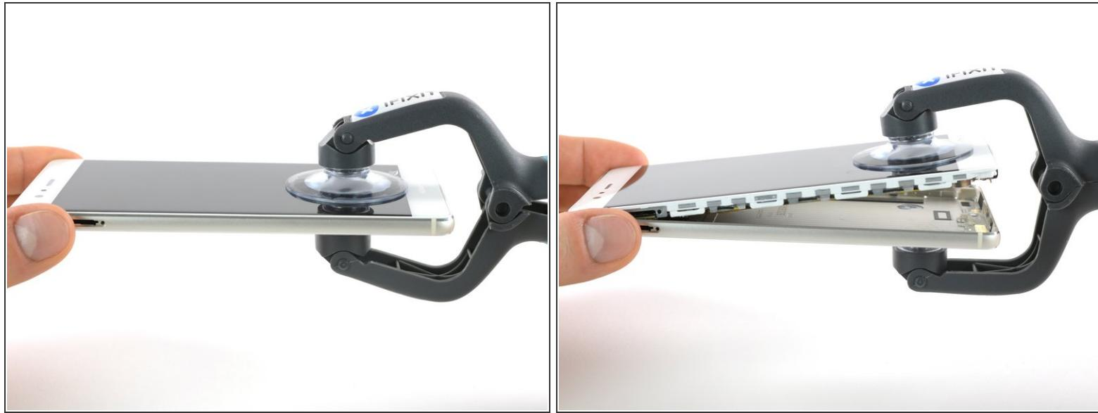
**⚠** Avoid to lift only the display instead of the whole phone assembly as doing so may cause damage to the screen.
